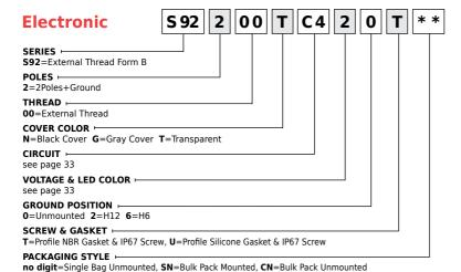
mPm® Field Attachable DIN Valve Connectors
