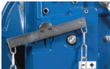
Remote Lock Cam and Lever attached to Chains
