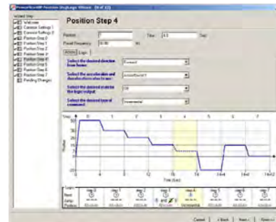
StepLogic wizards available for ease of position or velocity StepLogic programming using drive software tools.
