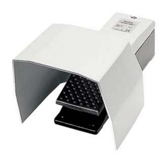
LATCHING FOOT OPERATING SWITCH, SINGLE PEDAL M20X1,5 CABLE ENTRY IP65, 1NO + 1NC, WITH COVER
