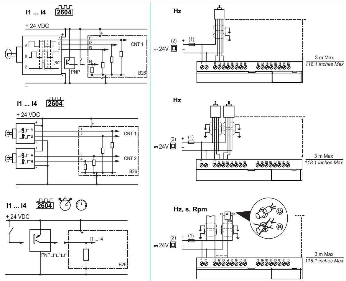
(1) 1 A (UL248) quick-blowing fuse, circuit-breaker or circuit protector (US)
