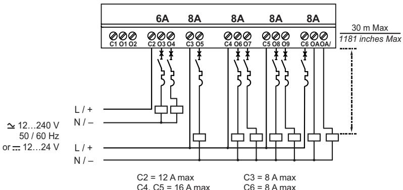
(1) 1 A (UL248) quick-blowing fuse, circuit-breaker or circuit protector (US)
