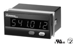
The Codix 541 is a voltage powered pulse counter / position display with 4 count input modes: count direction, difference, addition, quadrature (phase discriminator) x1, x2 and x4, for fast and slow count pulses, with 6-digit LED display for NPN, PNP input signals.
