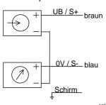
Pin configuration of connector M12x1 (4-pin) /
