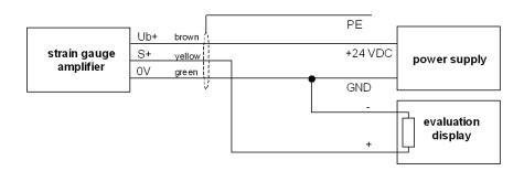
Pin assignment for cable integrated amplifier
