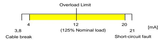
Adjusting the signal shift to 8 mA after activating the test relay the overload limit is overtraversed in every operating status. But as the upper range limit of 20 mA isn't reached its possible to check the signal swing.
