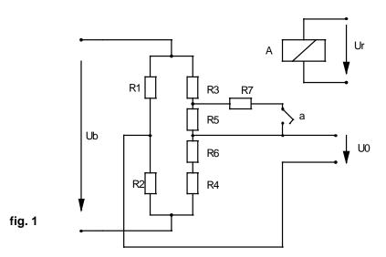
Applying R7 causes a defined, static detuning of the zero point (diagonal voltage) of the whatstone-bridge. Using an extern control, which is independend of the load cell (because of security reasons it has to have 2-channels), it's possible to activate the relay A and to change the output signal of the load cell in a defined way.
