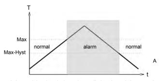
switchover delay time  $(t_{\mbox{\scriptsize DS}})$  can be applied to the switchover to the alarm state. Equally, one switch-back delay time (t<sub>DR</sub>) of several can be applied to switching back to the normal state.
