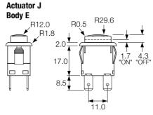
Spacing between centre of terminals 1 & 3 or 2 & 4 is 10.0mm
