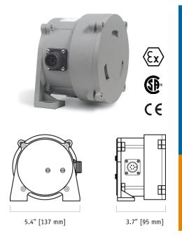
The model IT9420 is a rugged yet simple device which provides a 4 to 20 mA current feedback signal for incline position. The heart of the IT9420 is a magnetically-damped pendulum coupled to a conductive plastic precision potentiometer. A highly linear relationship between inclination and a 4 to 20 mA output is maintained over the full range of the IT9420.
