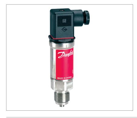
The standard heavy duty pressure transmitter MBS 4050 with integrated pulse-snubber is designed for use in industrial applications with severe media influences like cavitation, liquid hammer or pressure peaks and offers a reliable pressure measurement, even under harsh environmental conditions.
