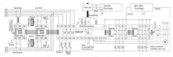
MSR300 system with various inputs, Two Output Groups with common monitored reset (reset alternative via DeviceNet with S34 linked to Y34), Group 1 with monitored contactors Safety Mat or E-Stop shut down both Output modules, Safety Gates only shut down the Group 2 module.
