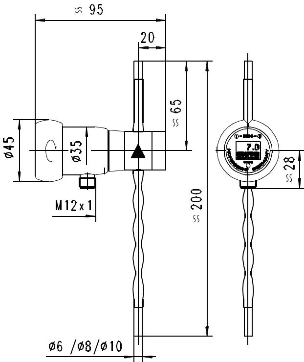
A spacer between the electronics head and the medium-contact measurement tube provides thermal decoupling between the two units. The media temperature may be raised for 45 min. to 130 °C.
