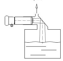
High dust levels reduce the ultrasound signal and produce incorrect measurements. Depending on density, foams may or may not be recognised.
