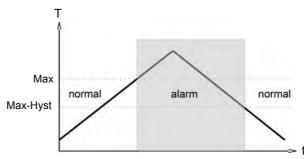
The change to the alarm state is indicated by the integrated red LED and a cleartext in the display. While in the normal state the switching outputs are at the level of the supply voltage; in the alarm state they are at 0 V, so that a wire break would also display as an alarm state at the signal receiver.
