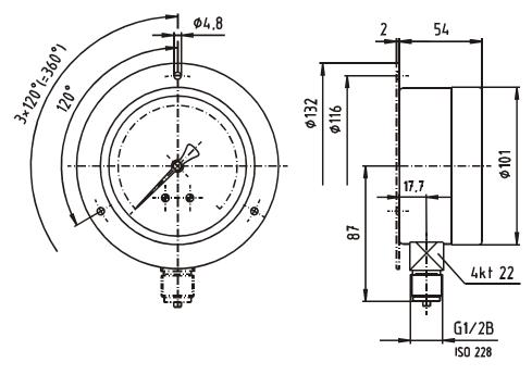
Model P2324 / P2325 hole pattern for front and rear flanges
