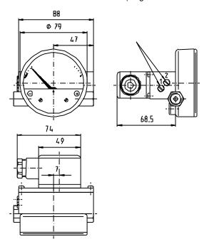
Switching point by means of adjustable spindle from the outside over a range of 10% to 100% of the full scale value.
