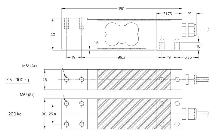
PC1: Mounting bolts M6 8.8; torque 10 Nm. Torque value assumes oiled threads.
