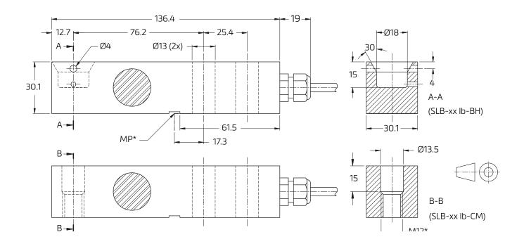
Mounting bolts for 200 lb to 2500 lb: M12 8.8 / torque 90 Nm; for 5000 lb: M12 10.9 / torque 120 Nm. Torque values assume oiled threads.
