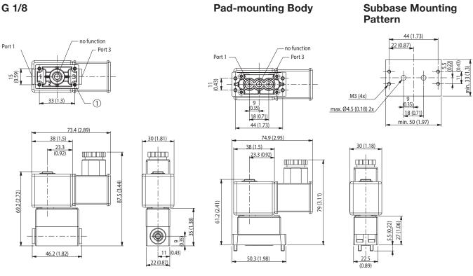
4 mounting holes, max. depth 7mm (0.276in), for self-tapping screw (type EJOT PT, K30)
