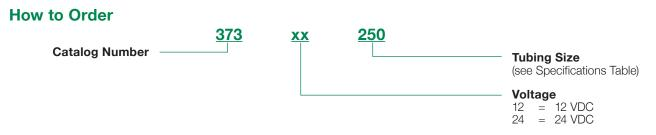
Ordering Example: 37312430 = 1.60mm (0.063in) x 4.8mm (0.188in) tubing, 12 VDC, 2.07 bar (30 psi) max
