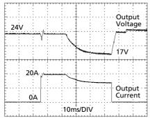
20A Peak load (resistive) for 50ms Output voltage dips from 24V to 17V.
