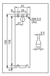
Fig. 24-6 Wall/panel mounting, side view
