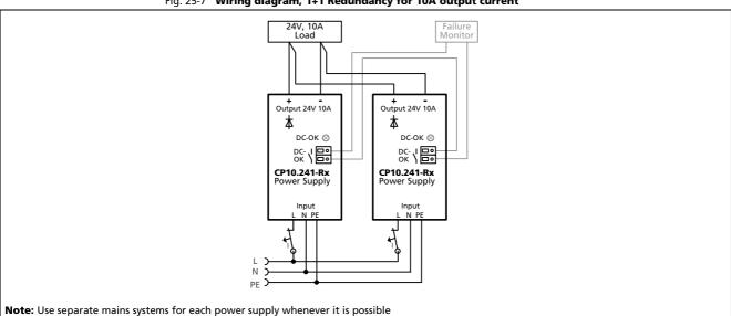
Fig. 25-7 Wiring diagram, 1+1 Redundancy for 10A output current
