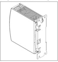
Fig. 24-4 **Wall/panel mounting, front view**
