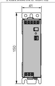
Fig. 24-5 Hole pattern for wall mounting
