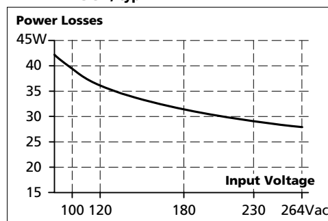
Fig. 9-4 Losses vs. input voltage at 36V, 13.3A, typ.
