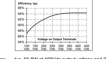
Full-load Power Losses: typ. 60.8W at 400Vdc output voltage and 2.6A output current
