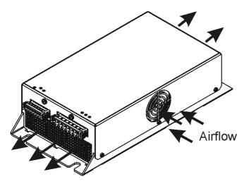
The fan will only run if needed during high temperatures. The fan will also run for 8 seconds after applying sufficient input voltage. This allows to check the function of the fan. Furthermore, the fan will run approximately every three hours for a short time to avoid a stiffness of the fan after long breaks and to extend the life of the fan.
