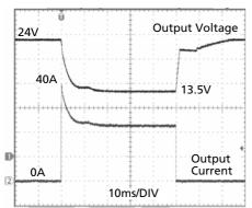
40A Peak load (resistive) for 50ms Output voltage dips from 24V to 14V.
