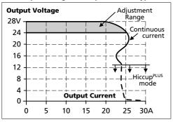
Fig. 6-2 **Short-circuit (50mOhm) on output, Hiccup<sup>etus</sup> mode, typ.**
