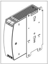
Fig. 20-2 Side mounting with DIN-rail brackets
