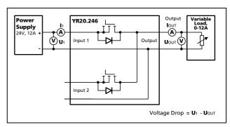
Fig. 21-4 Test setup for power loss measurements
